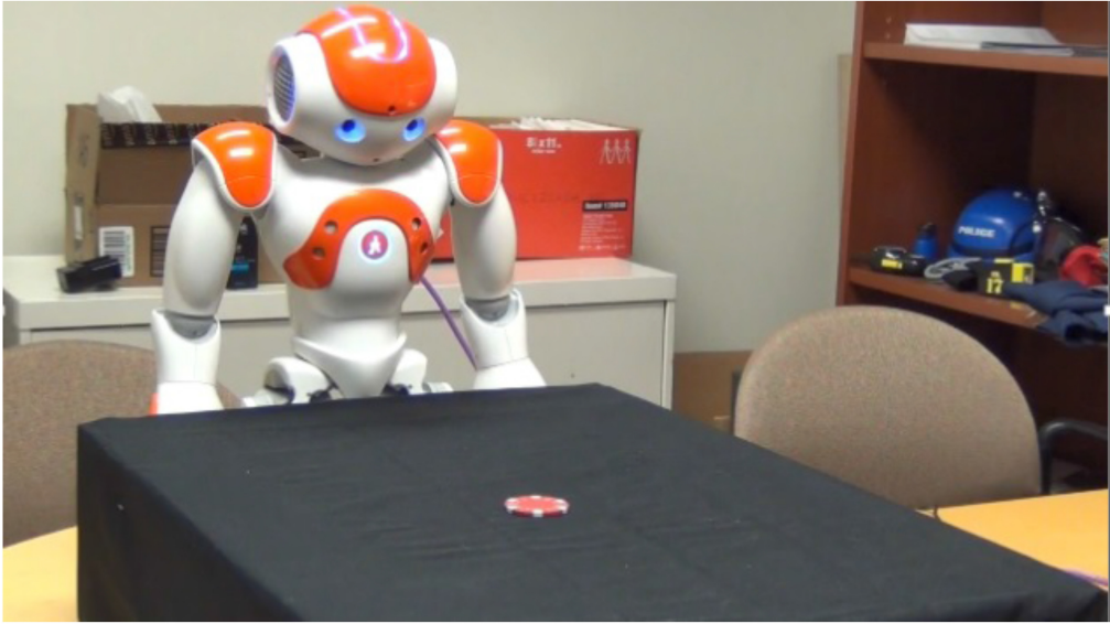
Fig. 6. The figure depicts a NAO robot playing the Investor-Trustee game with a human. The robot plays the role of investor using an evolving model of the person to predict their response to a particular investment.
