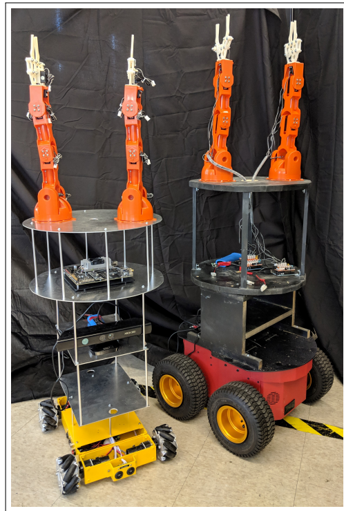
Fig. 9. Image of the guide robot prototypes. These robots are currently being built for future use in physical experiments. The arms of the robot gesture to communicate guidance directions.
