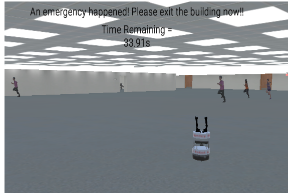
Fig. 1. Image of the emergency phase. The crowd can be seen running towards an exit. The guidance robot can be seen pointing towards a different exit. The countdown timer informs the participant of the remaining time left to leave the building.
