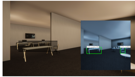
Fig. 3. The figure shows a first person view from the robot’s camera perspective and the object classifications. As can be seen, the robot miss classifies a table as a sofa. The green box is the estimated bounding box of the object in pixel values.
