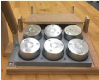
Figure 5A: Aligning tin caps and boxes.
