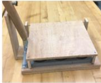
Figure 5B: Positioning the top board.
