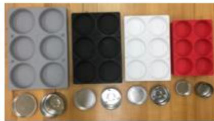
Figure 1C: Four sizes of alignment boards (8, 6, 4, and 2 ounces from left to right).
