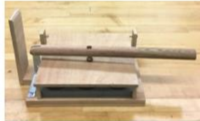
Figure 5C: Applying and distributing a point force to cap the tin boxes.
