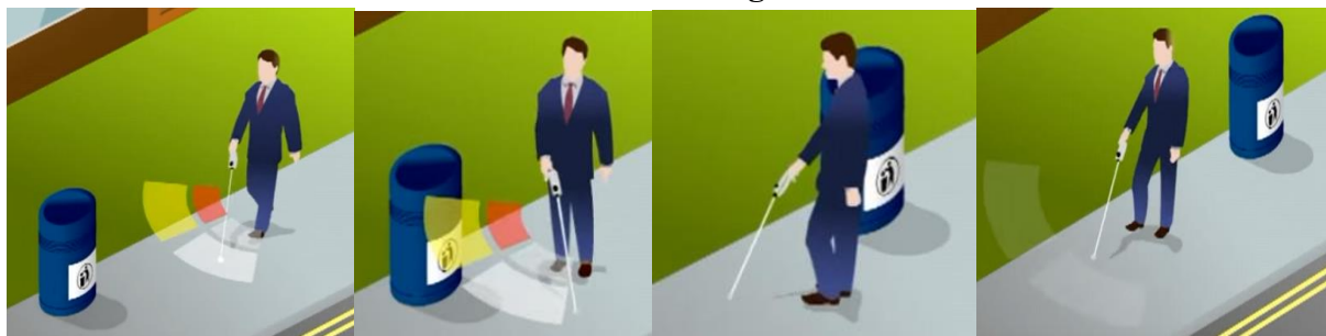
Figure 1: A visually impaired person using the sensor enabled white cane to avoid a trash can before encountering it.
