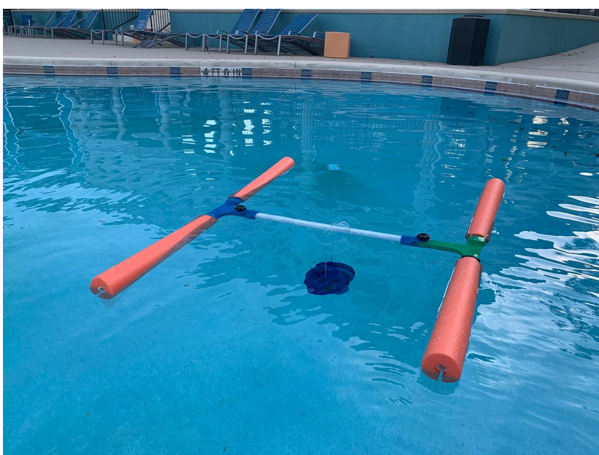
Figure 3: The primary frame and buoys were tested for buoyancy in a swimming pool. The device was able to support a maximum of 36 lbs. Underwater, an average X year old's weight with buoyancy forces under consideration is 13.12 lbs, assuming the position of the X year old is half above water and half underwater due to the position of the board relative to the middle support. Based on the volume of the plates used, each plate provides a net force down of approximately 4 lbs; at 9 weights plates, the device failed, demonstrating that it supports up to 2.6 times the weight of the average X year old.
