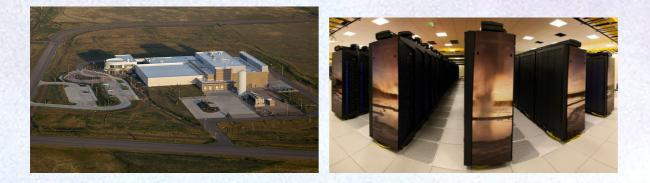
$\approx$ 72K cores = 4536 (nodes)  $\times$  16 (cores) and each core with 2Gb memory 16 Pb parallel file system
