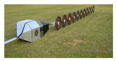
boom beneath the helicopter. The company has been safely using aerial tree-trimming since 1988 and aerial saws are in accordance with American National Standards Institute (ANSI) A300 tree pruning standards.
