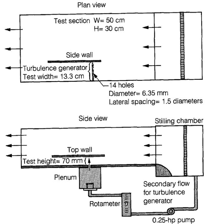
Fig. 1. Plan view (top schematic) and side view (bottom schematic) of the water channel facility used for the initial development of the turbulence generator
