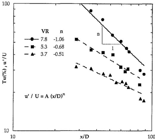
Fig. 2. Streamwise turbulence intensity decay as measured in the water channel tests comparing velocity ratios
