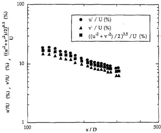
Fig. 7. Streamwise decay of turbulence for streamwise, vertical, and combined fluctuating velocities
