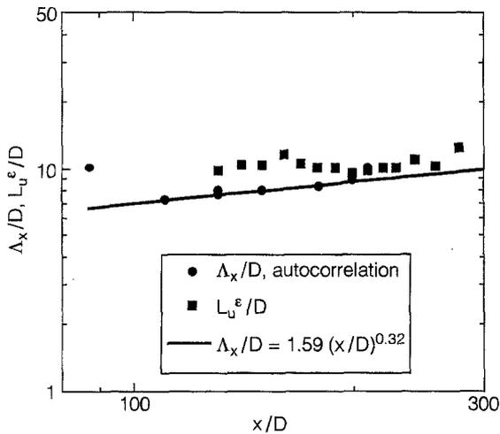
Fig. 8. Streamwise integral and dissipation turbulent length scales for the high turbulent flow field
