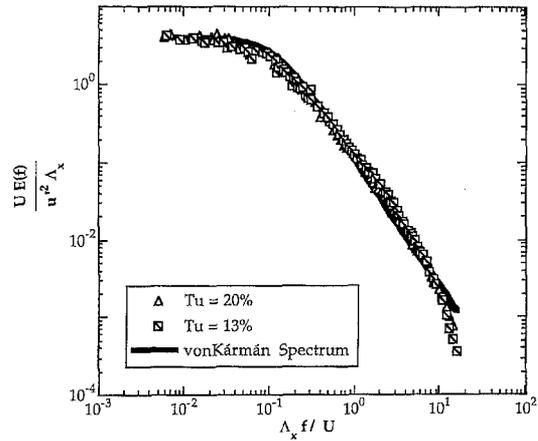
Fig. 9. Energy spectra of freestream turbulence as compared with the vonKármán Spectrum
