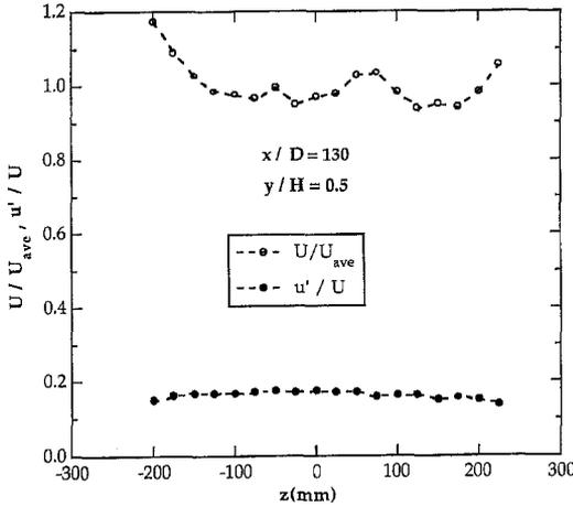
Fig. 4. Spanwise uniformity of highly turbulent flowfield at the mid-height of the tunnel and at a downstream distance measured from the jets of  $x/D=130$
