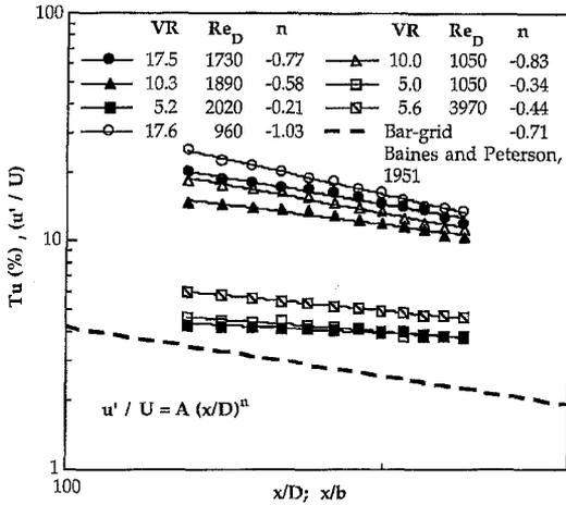
Fig. 5. Streamwise decay of turbulence levels as a function of jet-to-mainstream velocity ratio and jet Reynolds number as compared with grid-generated turbulence
