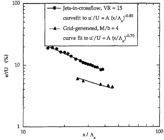
Fig. 6. Streamwise decay of turbulence compared with grid-generated turbulence. Streamwise distance is normalized by the integral length scale
