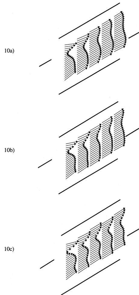
Fig. 10. Measured mean velocity vectors progressing through the fifth louver passage at: (a)  $Re = 230$ ; (b)  $Re = 450$ ; and (c)  $Re = 1016$ .
