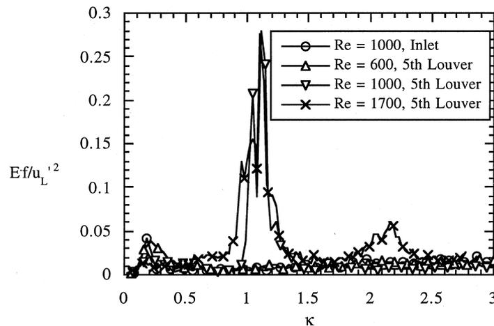
Fig. 12. Energy spectra versus wave number for measured velocity fluctuations at the inlet and downstream of the fifth louver for a range of Reynolds numbers.
