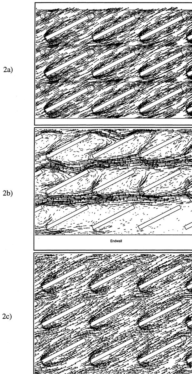
Fig. 2. CFD predictions showing differences in the flowfield for: (a) periodic boundary condition model; (b) 5 row model; and (c) 19 row model.
