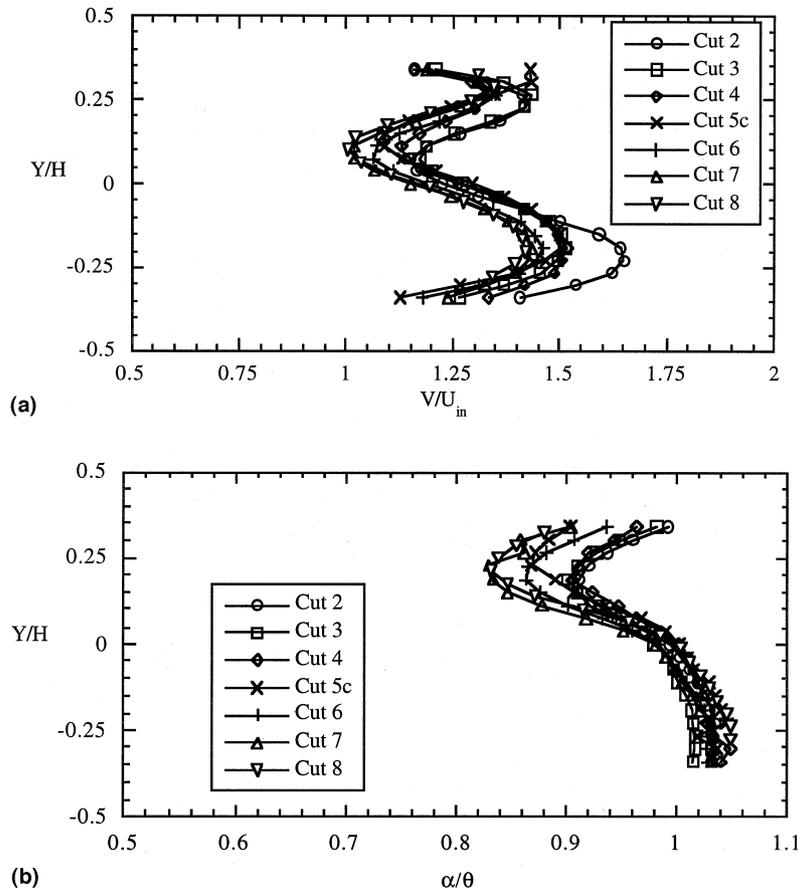
Fig. 8. Mean velocity measurements progressing streamwise through louver passages at  $Re = 230$  showing: (a) normalized velocity magnitude; and (b) ratios of flow to louver angle.
