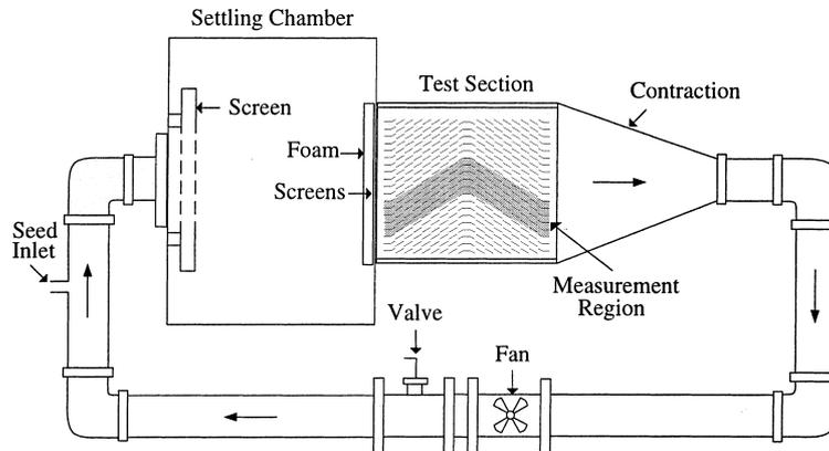
Fig. 3. Flow loop for velocity measurements in the large-scale model.
