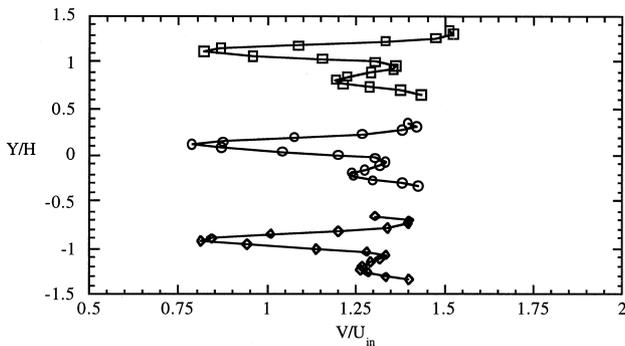
Fig. 5. Measured mean velocity magnitudes in three adjacent louver passages at  $Re = 1016$ .
