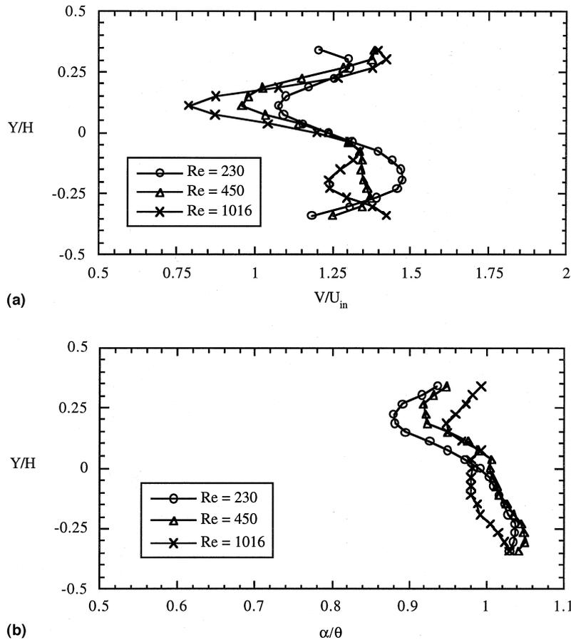
Fig. 9. Mean velocity measurements at cut 5c indicating Reynolds number effects on: (a) normalized velocity magnitude; and (b) ratio of flow angle to louver angle.
