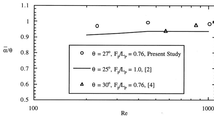
Fig. 6. Measured ratios of average flow angle to louver angles as a function of Reynolds number in the fifth louver passage compared with prediction by Achaichia and Cowell [2] and measurements by Webb and Trauger [4].
