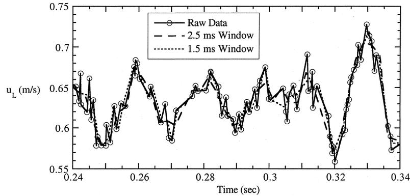
Fig. 11. Example of raw velocity measurements downstream of the fifth louver compared with equally-spaced velocities using two window sizes over a small time period at  $Re = 1000$ .
