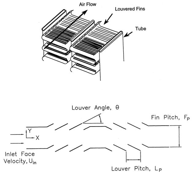
Fig. 1. (a) and (b) Illustration of the louvered plate fin heat exchanger and important parameters for the finned louver geometry.
