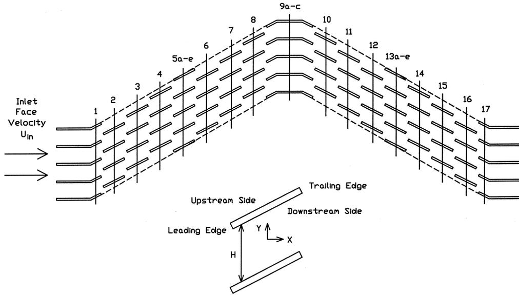
Fig. 4. Detail of measurement region showing cut locations of velocity profile measurements and louver terminology.
