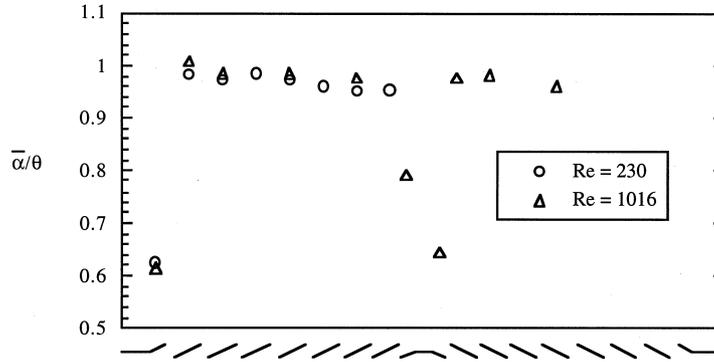
Fig. 7. Streamwise progression of measured average ratios of flow angle to louver angle at two Reynolds numbers.
