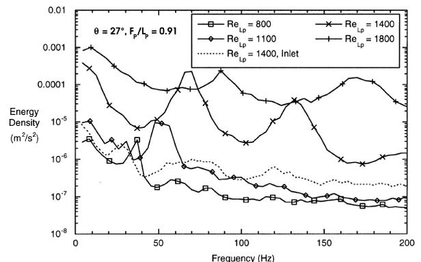
Fig. 12. Spectra of the velocity fluctuations downstream of a fully developed louver for  $\theta = 27^\circ$  and  $F_p/L_p = 0.91$ .
