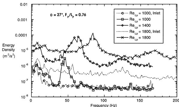
Fig. 11. Spectra of the velocity fluctuations downstream of a fully developed louver for  $\theta = 27^\circ$  and  $F_p/L_p = 0.76$ .
