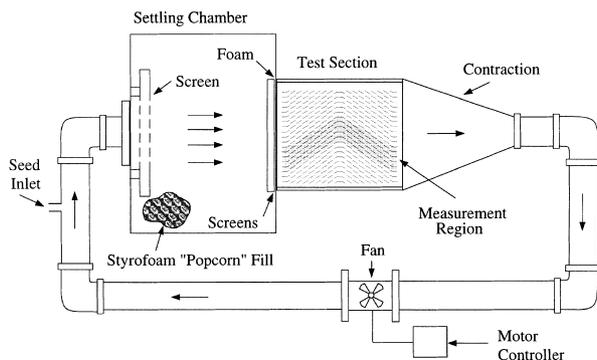
Fig. 2. Experimental test set-up with 20:1 scaled-up louver models.
