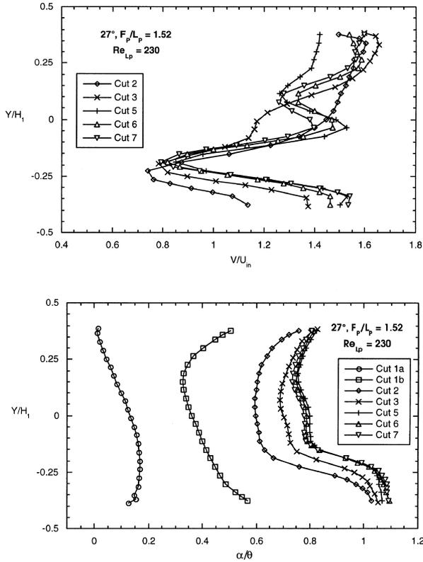
Fig. 6. (a), (b) Velocity magnitude and flow angle profiles showing development through the louver bank for  $\theta = 27^\circ$  and  $F_p/L_p = 1.52$  at  $Re_{Lp} = 230$ .
