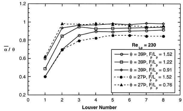
Fig. 9. Effect of fin pitch and louver angle on the average flow angle progressing through the louvers for  $Re_{Lp} = 230$ .
