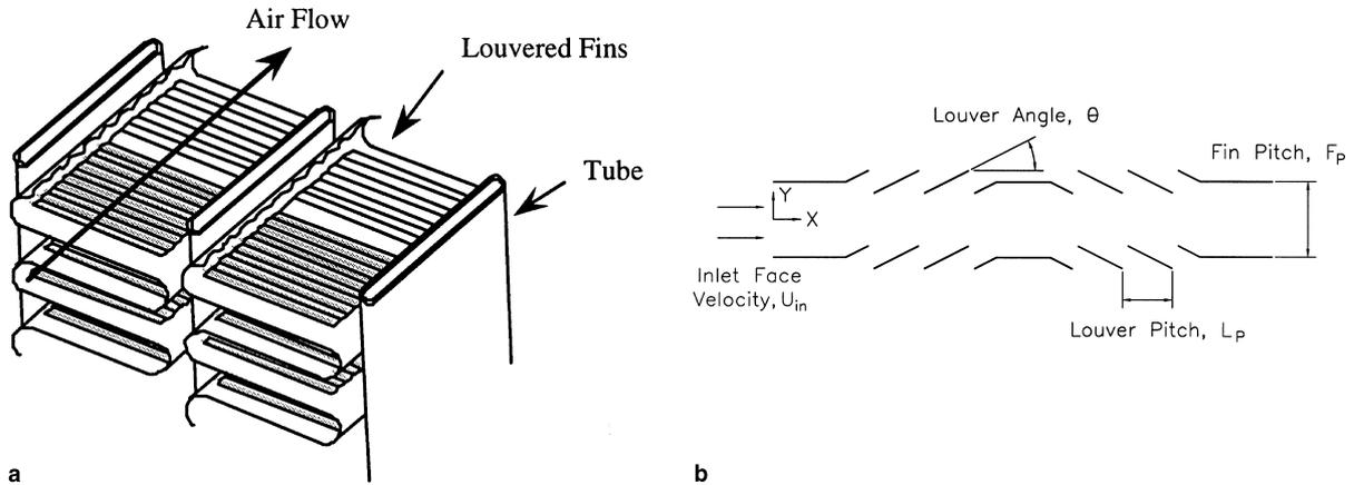
Fig. 1. (a) Schematic of louvered fin-and-tube heat exchanger. (b) Illustration of the geometrical parameters of interest for a louvered fin.
