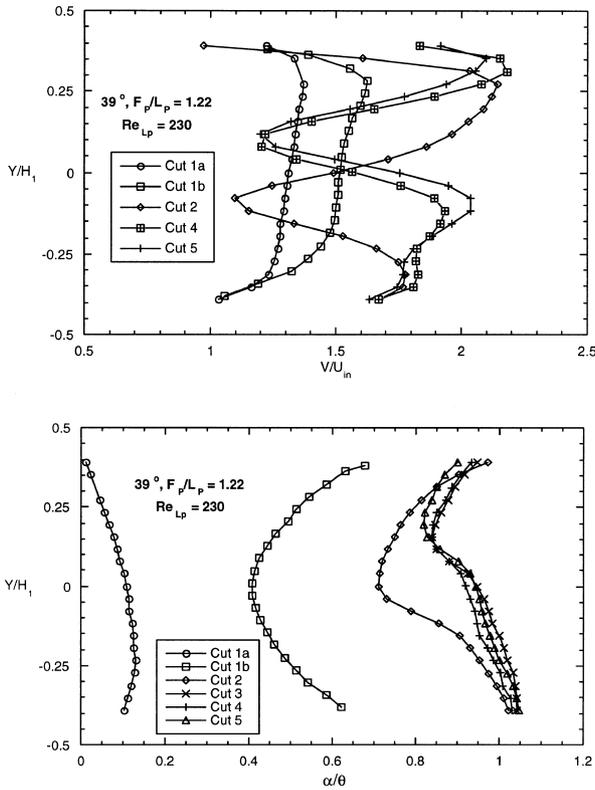
Fig. 8. (a), (b) Velocity magnitude and flow angle profiles showing development through the louver bank for  $\theta = 39^\circ$  and  $F_p/L_p = 1.22$  at  $Re_{Lp} = 230$ .
