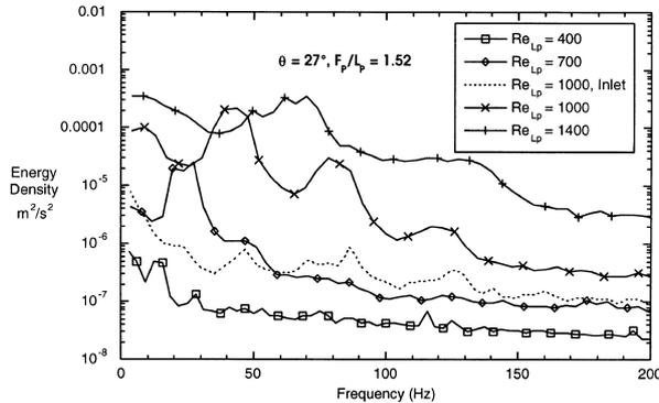
Fig. 13. Spectra of the velocity fluctuation downstream of a fully developed louver for  $\theta = 27^\circ$  and  $F_p/L_p = 1.52$ .
