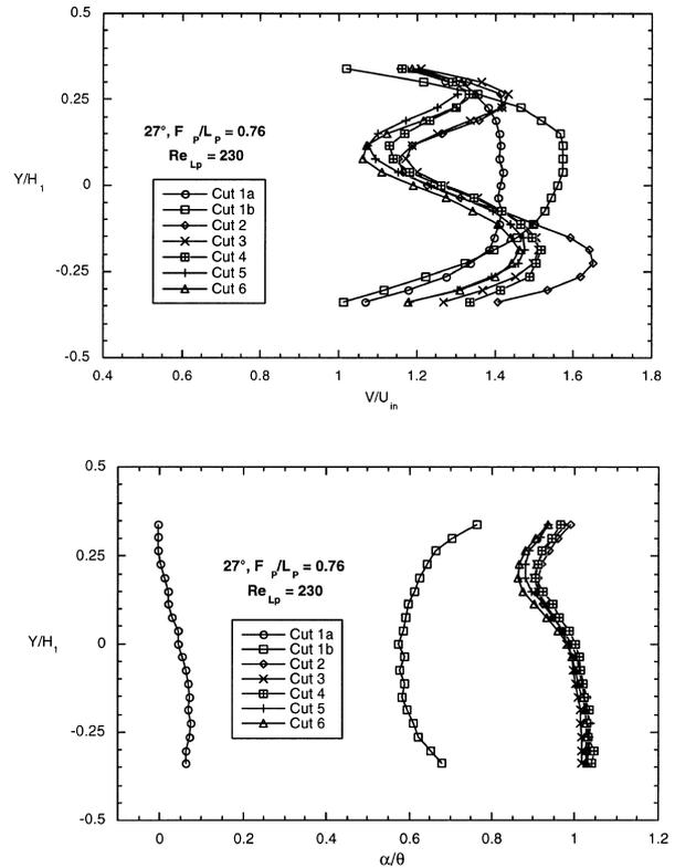
Fig. 4. (a), (b) Velocity magnitude and flow angle profiles showing development through the louver bank for  $\theta = 27^\circ$  and  $F_p/L_p = 0.76$  at  $Re_{Lp} = 230$ .
