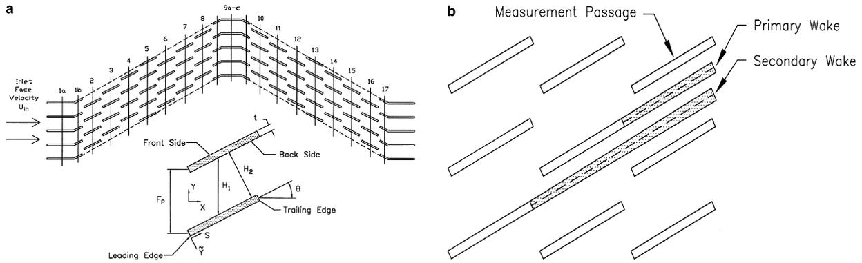
Fig. 3. (a) Locations of measurement cuts for bulk flow in the louver passages. (b) Illustration of the primary and secondary wake terminology.
