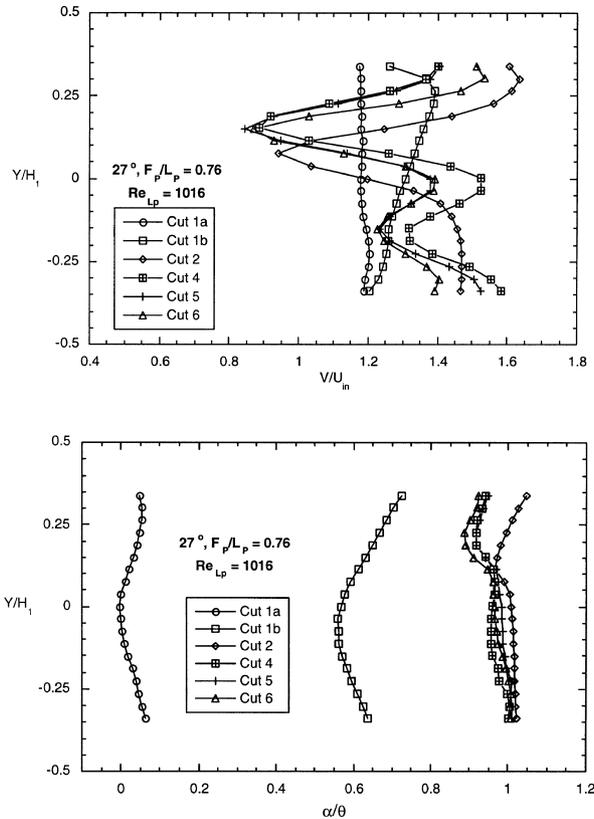
Fig. 5. (a), (b) Velocity magnitude and flow angle profiles showing development through the louver bank for  $\theta = 27^\circ$  and  $F_p/L_p = 0.76$  at  $Re_{Lp} = 1016$ .
