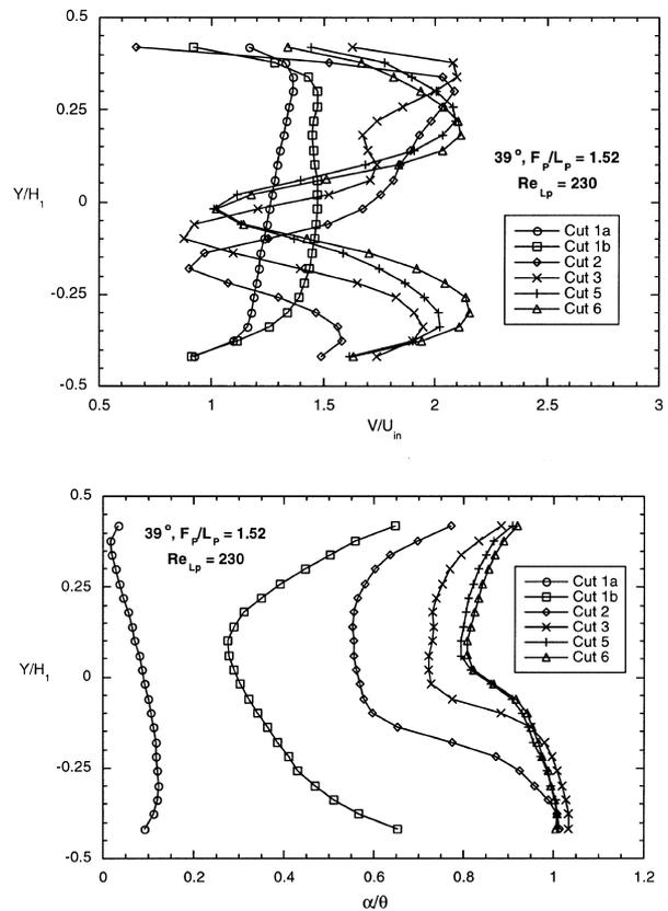
Fig. 10. (a), (b) Velocity magnitude and flow angle profiles showing development through the louver bank for  $\theta = 39^\circ$  and  $F_p/L_p = 1.52$  at  $Re_{Lp} = 230$ .
