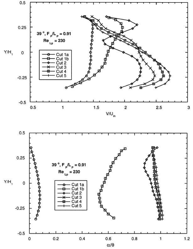
Fig. 7. (a), (b) Velocity magnitude and flow angle profiles showing development through the louver bank for  $\theta = 39^\circ$  and  $F_p/L_p = 0.91$  at  $Re_{Lp} = 230$ .
