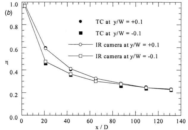
**Fig. 14** Adiabatic effectiveness contours (a) and downstream levels (b) on the endwall for the case with dilution jets
