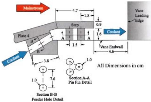
Fig. 4 Schematic illustrating the combustor liner exit slot
