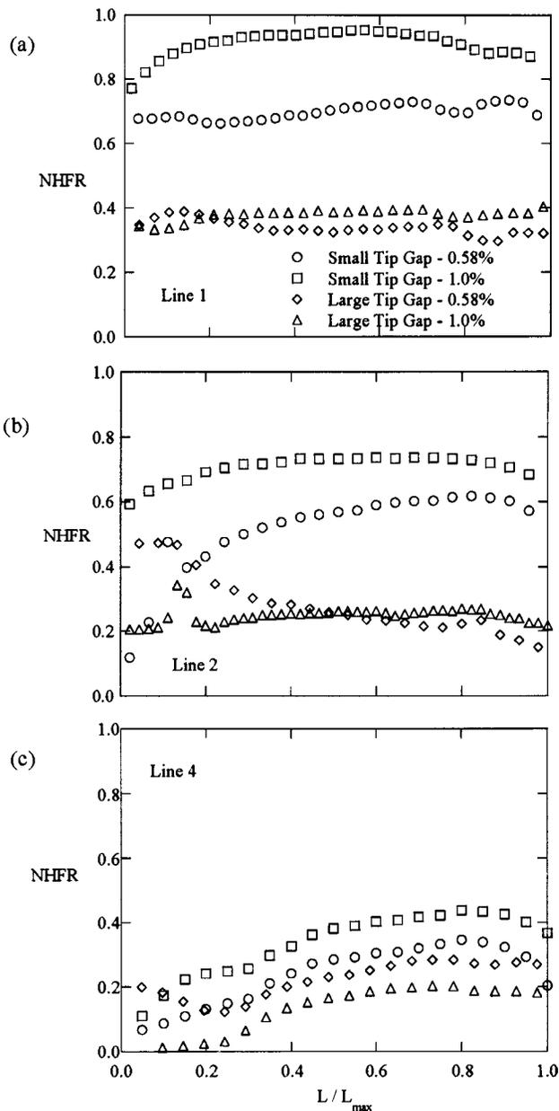
Fig. 14 (a)–(c) Individual line plots of NHFR at different locations along the blade tip
