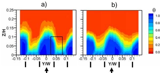
Figure 7a, b. Thermal field measurements for plane 2p for (a) case 2, (b) case 3. The black rectangle in 8a denotes where the flow field of Figure 9 was measured.
