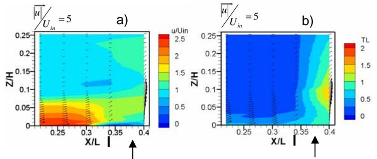
Figure 9a, b. (a) Flow field at plane 1s for case 1. Vectors show  $u/U_{in}$  and  $w/U_{in}$  velocity components and contour shows  $u/U_{in}$  values. (b) Flow field vectors and contour of turbulence level at plane 1s for case 1.
