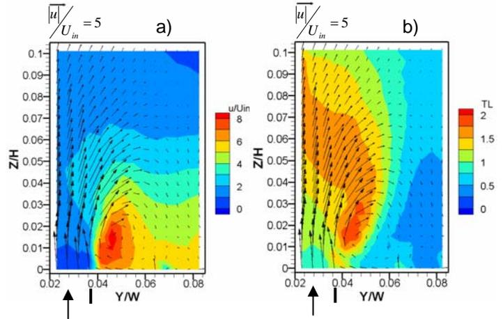
Figure 8a, b. Vectors show  $v/U_{in}$  and  $w/U_{in}$  velocity components. (a) Flow field at plane 2p for case 1 with contours showing  $u/U_{in}$  values. (b) Contour of turbulence level at plane 2p for case 1. Note 4x enlargement of scale.
