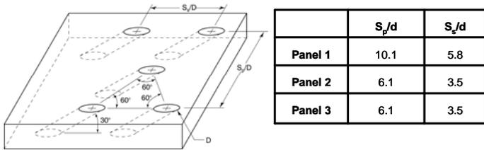
**Figure 2b. Illustration and description of cooling hole arrangement for liners.**
