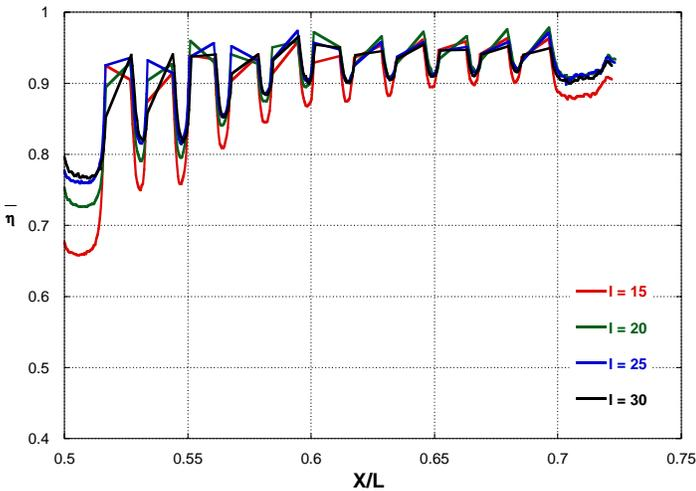
Figure 5. Adiabatic effectiveness profile for four film-cooling blowing ratios at the dilution center-line.
