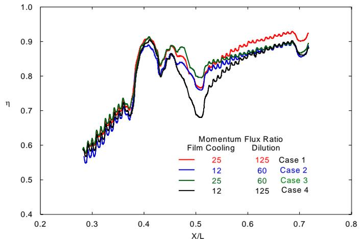
**Figure 4. Lateral average of adiabatic effectiveness for all cooling configurations.**
