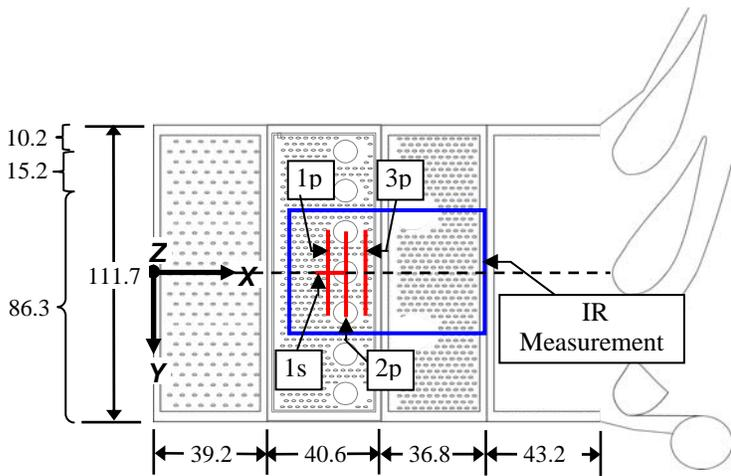
**Figure 2a. Layout and measurements planes for the combustor simulator (dimensions in cm).**
