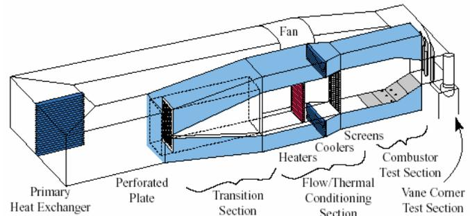
**Figure 1. Illustration of the wind tunnel facilities used for combustor simulator experiments.**
