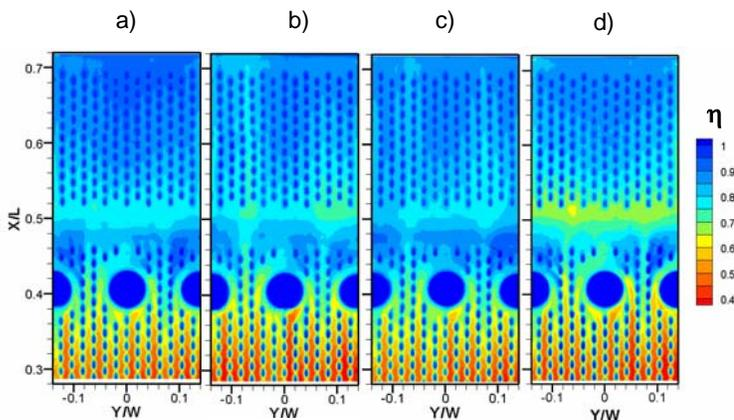
**Figure 3a-d. Adiabatic effectiveness contours for (a) configuration 1, (b) configuration 2, (c) configuration 3, and (d) configuration 4.**
