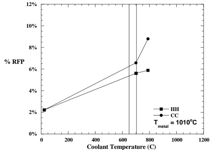
**Figure 18. Operating at higher coolant temperatures increases %RFP (0.5 grams, ISO Fine 60-hole coupon, Tmetal = 1010°C).**
