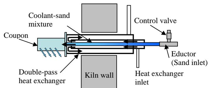
Figure 3. The test rig for the sand ingestion tests included a sand delivery system.
