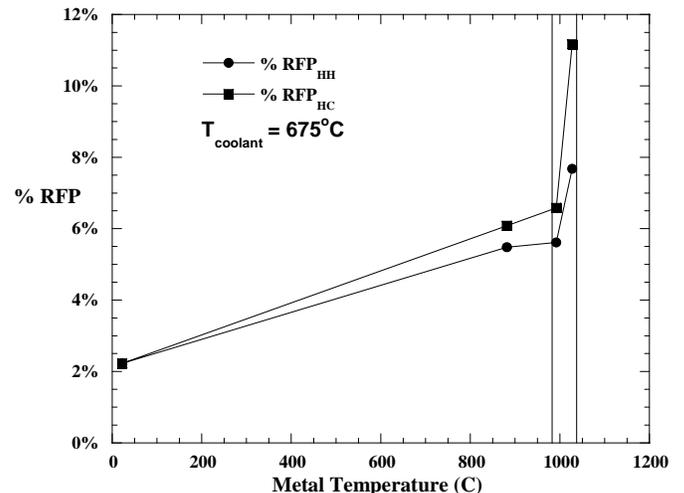
**Figure 19. Metal temperature over 1000 °C can cause significant enhancement of %RFP (0.5 g ISO Fine, 60-hole coupon, Tcoolant = 675°C).**
