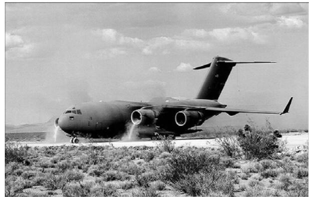
Figure 1. Sand ingested into a C-17 during takeoff.
