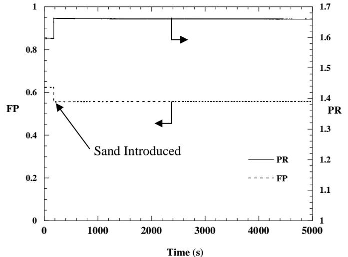
**Figure 7. The flow parameter and pressure ratio stabilize a few seconds after sand is introduced and remain steady.**
