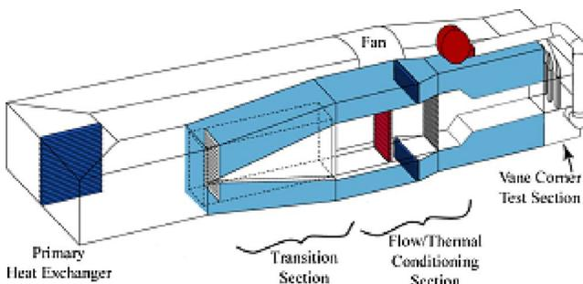
**Fig. 3 Illustration of the wind tunnel facility**
