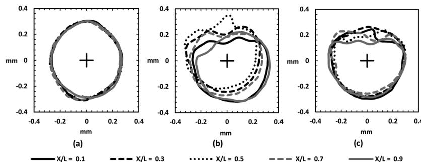
**Fig. 8 Axial slices at various streamwise locations of (a) vertically, (b) horizontally, and (c) diagonally built channels**
