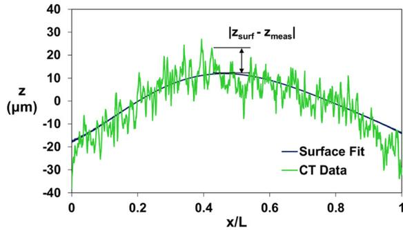
Fig. 4 A slice taken along the channel axis showing the roughness features and surface fit for one plane of the vertically built channel surface
