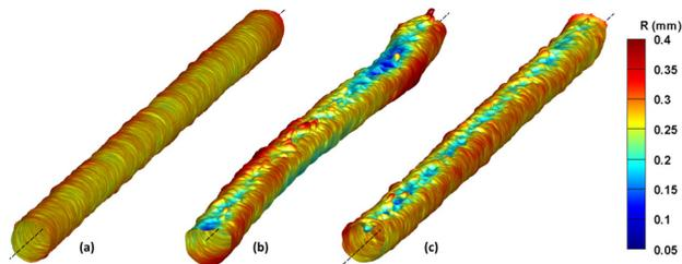
**Fig. 7 Three-dimensional surfaces representing the internal channel topology of a single channel for the (a) vertical, (b) horizontal, and (c) diagonal build directions**
