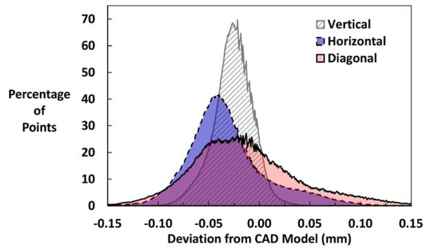
Fig. 6 Distribution of the difference between the coupon surface points and the CAD model for the three different build directions
