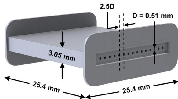
Fig. 1 Designed dimensions, shape, and channel spacing of the test coupons
