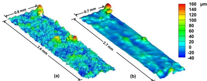
Fig. 5 Comparison of surface roughness contours from (a) an optical profilometer and (b) a CT scanner showing features missing in CT scan data
