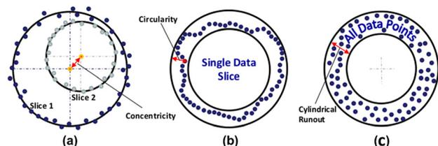
**Fig. 3 Geometric tolerance definitions for (a) concentricity, (b) circularity, and (c) total runout**
