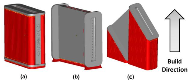
Fig. 2 Coupon orientation and support structures (shown in red/darker gray) for the (a) vertical, (b) horizontal, and (c) diagonal build directions
