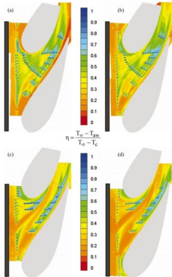
**Fig. 4 Contours of adiabatic effectiveness for the baseline film-cooling only cases: (a) pattern 1, 0.5% coolant (b) pattern #1, 0.75% coolant, (c) pattern #2, 0.5% coolant, and (d) pattern 2, 0.75% coolant**
