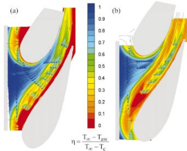
**Fig. 8** Predicted streamlines at 2% span for 1% slot without film cooling superimposed for (a) pattern 1 with 0.75% slot flow and 0.5% film cooling, and (b) pattern 2 with 0.75% slot flow and 0.5% film cooling
