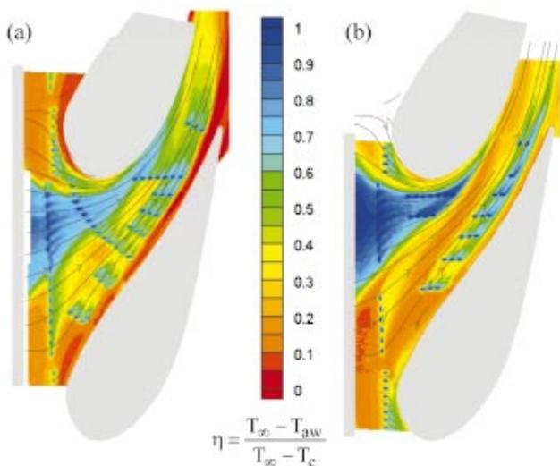
**Fig. 7** Predicted streamlines at 2% span for 0.5% slot flow without film cooling are superimposed on measured effectiveness levels for (a) pattern 1 with 0.5% slot flow and 0.5% film cooling and (b) pattern 2 with 0.5% slot flow and 0.5% film cooling
