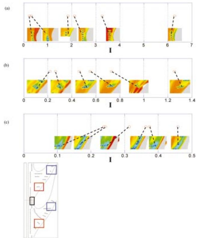
**Fig. 10 Momentum flux ratios for holes indicated by the dashed lines are shown in (a) leading edge, (b) pressure side upstream, and (c) pressure side downstream regions. Hole locations are shown to the right**
